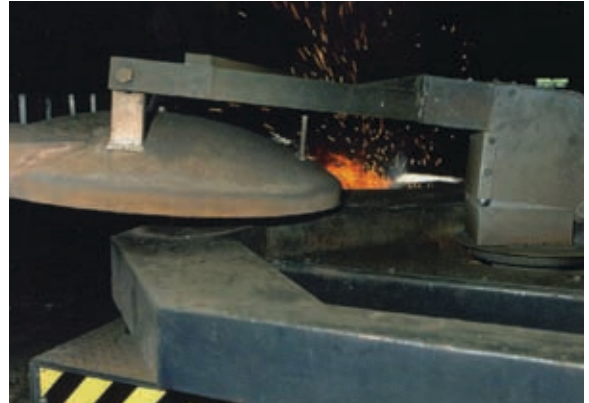
Properly managing the furnace lid is critical to energy savings.
