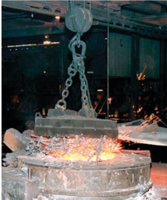
Overfilling overheats furnace components and allows heat to escape, wasting electrical power in two ways. It also jeopardizes safety, and is not recommended.
